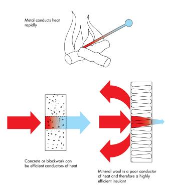
In relation to construction materials, metals are the best conductors of heat, followed by concrete and masonry. In contrast, wood and insulation materials are poor conductors, as are air and other gases.
