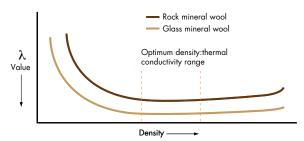
Each type of material has its own classic curve Glass mineral wool is more efficient at normal building temperatures than rock mineral wool
