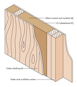
apparent that the insulation is bridged by the timber studs. In these circumstances, the combined method is appropriate.
