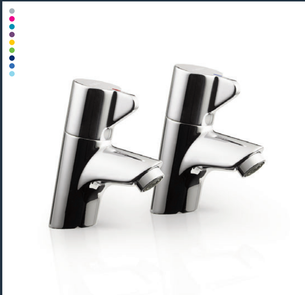
B8262AA Nuastyle 21 1/2" basin pillar taps (pair). Robust and durable, featuring anti-vandal outlets, these taps are perfect for use in public buildings and schools. Ergonomic quarter-turn handles control a ceramic disc cartridge and a laminar flow internal design minimises the risk of bacterial growth. Dual hot/cold indices are included and each tap is fitted with a 5lpm regulator (above).
