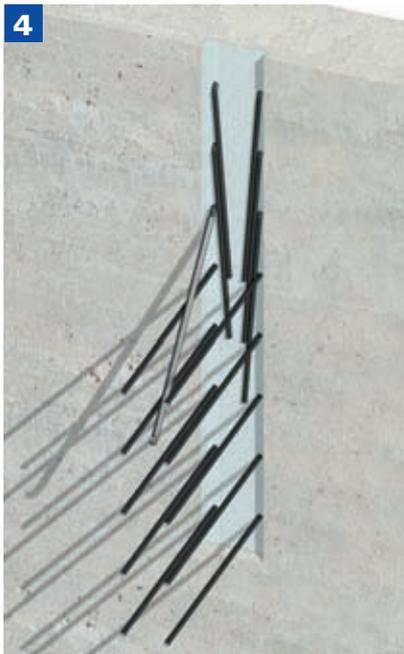
*Straighten the bars using the appropriate sized Ancon Eazistrip re-bending tool for the size of bar. The bars should be straightened only once. To avoid damage to adjacent concrete, it is prudent to allow a concrete curing period of seven days. See "Straightening of Bars" for more information.*
