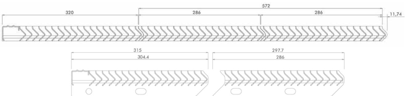
Flooring panels are framed either with a 34x4mm flat bar for laying on a steel section support or with a 60x4mm flat bar for side bolting.
