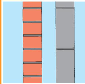
Most properties constructed during the past 100 years are constructed with cavity walls. A cavity wall consists of two skins of masonry. The inside skin is commonly of blockwork whilst the outside skin might be of brick, block or stone. It might also be of a rendered finish. The two skins do not touch one another but rise vertically maintaining a gap or 'cavity'.
