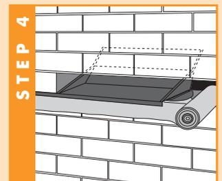
Take out another two bricks so you again have a three brick working space. Repeat the previous procedure until the run is completed.
