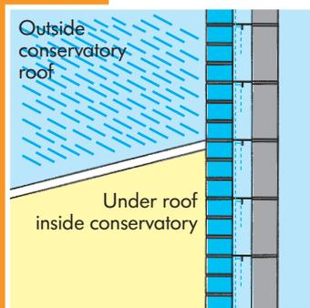
When a property is extended with a conservatory, the outside skin of the cavity wall becomes an inside skin below the new roof level. Wet and dampness can continue to gravitate and affect the wall, unless steps are taken to prevent it. The insertion of appropriate preformed cavity trays will stop the wet and dampness and the conservatory will stay dry.
