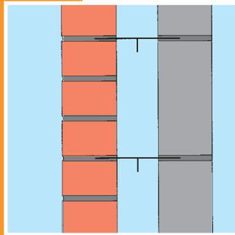
At regular intervals for stability, the two skins are tied together with wall ties. Such ties are designed to promote structural cohesion between the two skins. Ties are always shaped or twisted rather than being plain and flat. The reason for this is clear when heavy rainfall is experienced.
