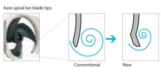
Escaping edges are sucked in by the bent blade edges, reducing overall turbulence.
