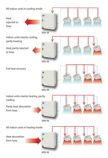
Heat recovery between outdoor units (Heat recovery and heat pump)
