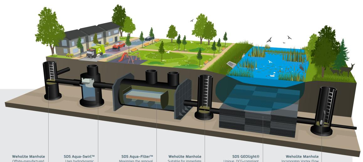
Offsite-manufactured, light weight HDPE, BBA HAPAS-certified manhole, available in multiple sizes and any orientation. Uses hydrodynamic, gravity-controlled separation technology to remove pollutants attached to silt and debris within surface water runoff. Maximises the removal of suspended solids such as nutrients, heavy metals and hydrocarbons and helps to reduce phosphorus.
