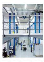
Vertical lift modules can go through several floors with up to six access openings placed on the front or rear side of the unit. A mezzanine floor can be installed to enable operation on several levels at the same time (with loading at one level or side and retrieval at the other).
