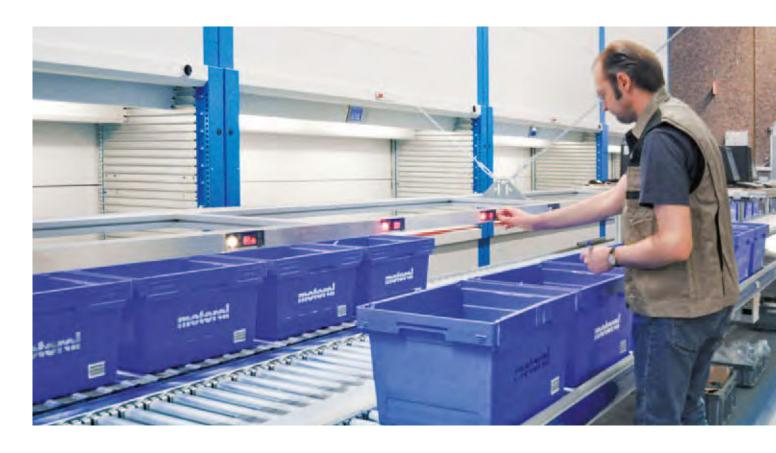
The amount of order picking locations and pick-by-light displays and the buffer capacity are determined by customerspecific demands.
