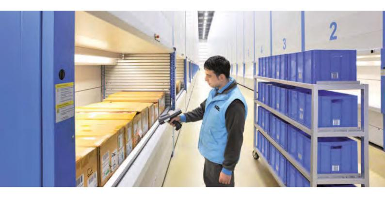
the picker is informed that the batch is completed. The picking cart with the bins is then taken directly to the next station or to the collection point.
