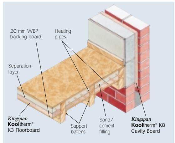
Figure 9 TIMBER FLOOR ON BATTENS
