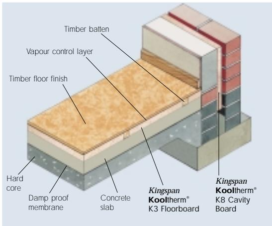
Figure 10 UNDERFLOOR HEATING - TIMBER FLOOR ON BATTENS
