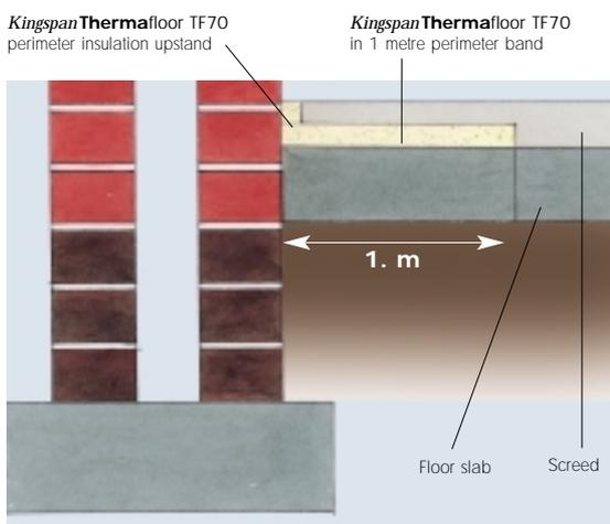
The greatest heat loss through an uninsulated floor is from the edges (Figure 4). Insulating the floor perimeter in a 1 metre band (Figure 5), will not only provide good insulating results but will also prevent the risk of cold bridging at the junction of the floor and external wall.
