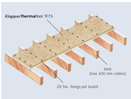
Boards should be fixed with nails/screws at 400 mm centres into all joists providing a minimum 25 mm penetration into the 50 mm wide joist (28 fixings per board). Do not nail within 25 mm from board corners.
