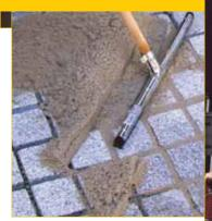
One component, ready-to-use polybutadiene-based drainage mortar for grouting paved floors with joints at least 5 mm wide subject to light stresses
