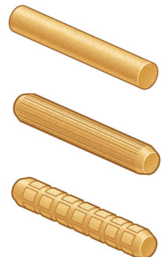
Smooth dowels are not recommended, grooved dowels are preferred
