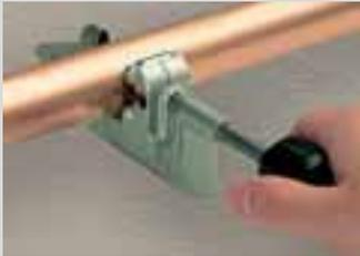
For copper tube, cut the tube square using a rotary tube cutter wherever possible, and for plastic pipe use pipe shears. Ensure the tube end is round and cut square.
