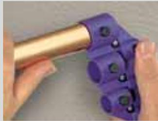
**2.** Remove any burrs or sharp edges from the external tube end using a T110 Multipurpose tool from the Tectite accessories range. Also ensure the internal bore is deburred and the tube is wiped clean and free of debris.
