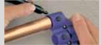
**5.** When using chrome plated copper tube you must scribe the tube using the T110 tool. Fully insert tube into the T110 and rotate twice whilst firmly pressing the button; check that the tube has been scribed.
