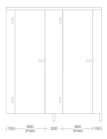
The cubicle door supplied in Box A measures 950mm (wide) and is to be cut-to-size on site. This cut is then concelaed by the full-height door hinge channel.
