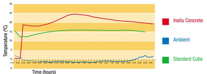
Figure 1- Highlights the difference in internal concrete temperature between the test cube and an insitu slab 300mm deep over the first 24 hours
