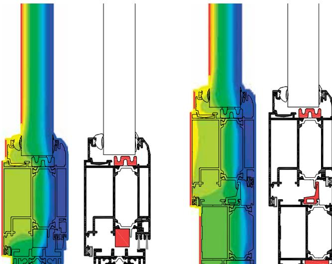
Metal Technology can provide tailored U-value calculations using their dedicated estimating software to calculate overall project average U-values for their full range of systems.
