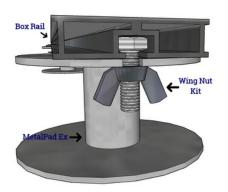
Utilising our <u>MetalPad Ex Class A Fire Rated</u> <u>Pedestals</u> with the M8 Wing Nut, which can be tightened by hand, offers significant benefits. This approach allows for the initial loose placement of pedestals and joists for precise positioning. Once in place, you can then securely tighten them to establish a stable and robust substructure system.
