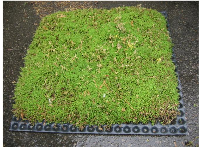
The whole idea is to provide as easy a way to install green roofs as possible. The modules are stacked onto pallets, for clean, fast delivery and making it easy to crane onto the roof. The modules can be stacked on top of each other up to 20 trays high onto a pallet for delivery to site. As the drainage sheeting is egg-box shaped, an air gap will maintain the vegetation for a **maximum of three days** before installation.
