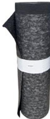
Permavent METAL uses the very high production methods of Permavent MAX as base layer to which a spiral layer of polypropylene mesh is melt bonded. It is specially design as a moisture and seperation layer for all types of standing seam and metal roofs. It is designed to be laid on top of rigid insulation or timber or plywood boarding and is clean, safe and lightweight.
