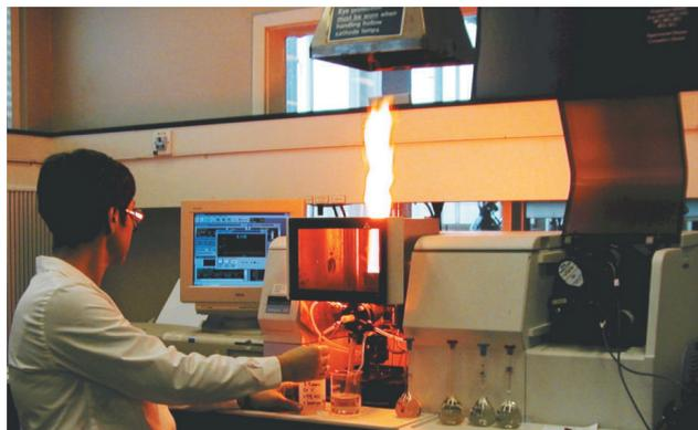
**AA spectrometer for trace element analysis**
