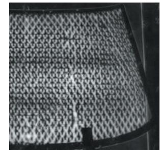
All glazings, whether Automotive or Architectural, require precise control of stress levels to ensure the product meets regulatory or environmental/robustness requirements. Various optical techniques are available to measure surface stresses, interior stresses and area stresses. Sometimes strain gauge technology is used to confirm that the product is able to withstand the thermal or mechanical stresses imposed by the glazing system.
