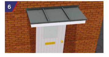
GRP Roof downstand to be fixed to GRP base using fir tree fixings as supplied. The upstand must be over flashed in lead or mastic sealed.
