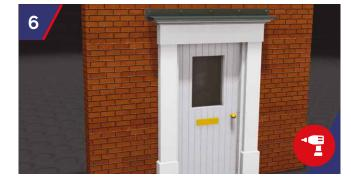
The pilasters are fixed to a timber battern running the full height of the pilaster and fixed into the reveal jamb if applicable. The upstand must be over flashed in lead or mastic sealed.
