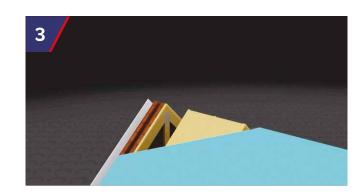
Apply roof felt over all of the roof including over the plywood panels. Only the area under the chimney needs to be felted during the lifting and fitting of the chimney. Lay the SmartStack chimney onto the roofing felt over the plywood panels, using the lifting eye situated within the SmartStack chimney pot.
