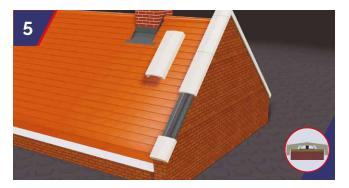
Clip all standard straight lengths between fixed junction units firmly pressing down onto fixing strip until "clicked" into position. If necessary, COPEKING® can be removed by gently prizing one side away from the wall until the holding down clip is released. Repeat for the other side. The white clips factory fitted internally to the COPEKING need to be fully located onto the fixing track as indicated in the above close-up.
