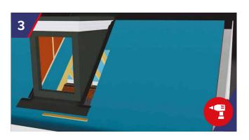
Fix timber cocking fillet to support lead. Lift GRP Dormer into place onto roof. Timber fillet can be positioned at a later date if the roof isn't being finished at the same time as the dormer installation.
