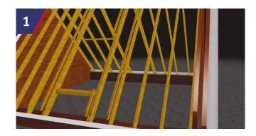
Trimming Rafters to be positioned under side cheeks with outer edge of outer most trimmer in line with GRP side cheek.
