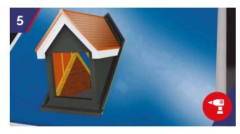
100mm x 75mm framing clamps screw fixed to side cheek framing and nailed or screw fixed to support rafters. Supplied and fitted by others, on site. Minimum of 3 No. per dormer side.
