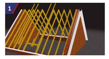
Trimming Rafters to be positioned under side cheeks with outer edge of outer most trimmer in line with GRP side cheek. Trimmers to be positioned 18mm below to the top of the trusses.
