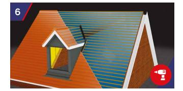
Battern out roof for tiling. Ensure the timber cocking fillet is installed creating a constant fall from the dormer onto the first row of tiles below the dormer. Using full and half tiles (tile and half preferred) set tiles within a maximum of 15mm from the side of the GRP dormer roof. This inside tile now covers the foam strip. Drill and nail all abutment tiles and adjacent tiles.
