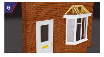
The roof will need to be insulated with suitable depth of quilt insulation prior to tiling the roof. Roofs can then be traditionally tiled and lead flashed to manufacturer's instructions.
