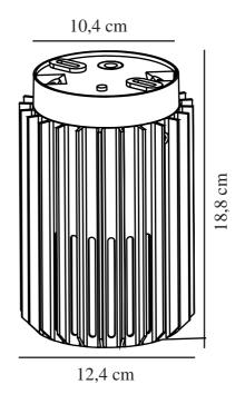
Voltage (V): 230 Volt IP degree: IP54 Maximum bulb wattage (W): 15W Class (Class 1, Class 2, Class 3): Class 1 (Earth contact) Socket type: E27 Parallel connection: True
