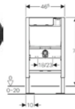
Geberit Duofix frame for wall-hung toilet, 79cm, with low-height furniture cistern
