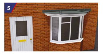
The window head is fixed to the GRP soffit using window manufacturers recommended fixings and sealed with suitable mastic joint.
