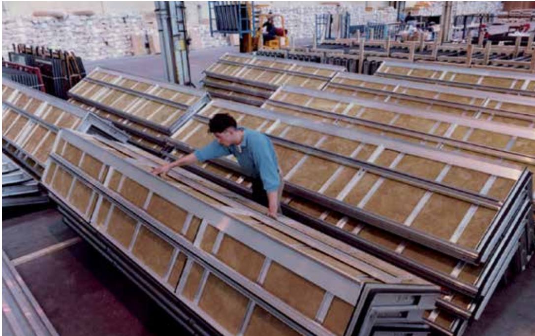
Unitised curtain walling corner panels being assembled in a factory.
