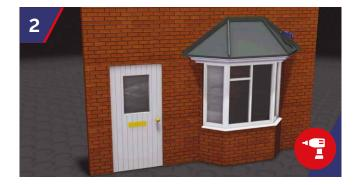
Using a 10mm drill bit, drill through the GRP Upstand into wall structure at a maximum of 450mm centres, to suit the StormFix 80 Fixing.
