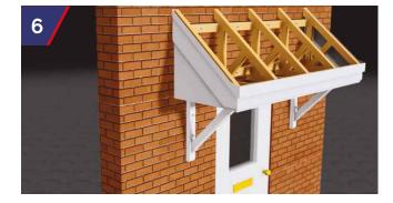
The Gallows Brackets are fixed to the canopy soffit in two places on each bracket. The Gallows Brackets are NOT to be used as the main structural support for the canopy. All tiling battens should be secured to all support trusses. The roofs can be traditionally tiled to manufacturer's recommendations.
