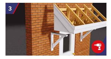
The canopy is placed on the brackets. Using a 10mm drill bit, drill through the rear structural timber truss into wall structure at a maximum of 450mm centres, to suit the StormFix 120 Fixing. Top and bottom rail running canopy length to be fixed back.
