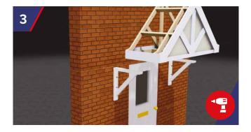
The canopy is placed on the brackets. Using a 10mm drill bit, drill through the rear structural timber truss into wall structure at a maximum of 450mm centres, to suit the StormFix 120 Fixing.
