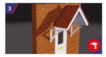
The canopy is placed on the brackets. Using a 10mm drill bit, drill through the GRP Upstand into wall structure at a maximum of 450mm centres, to suit the StormFix 80 Fixing.
