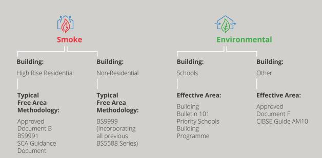
There are generally three methods to measure free area through a vent which are applied relative to the building type and the application (smoke or environmental ventilation).
