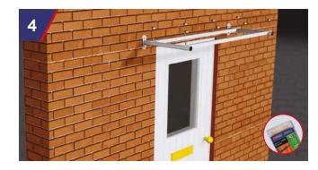
Place the plain bottom glass spacers and rubber washer seals onto each of the pole studs.
