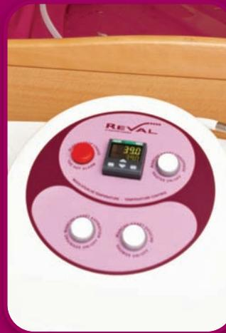
Position *Ruby* at the end of the bed and select temperature. Press the heater button and wait for *Ruby* to reach desired temperature (this takes approximately ten minutes from cold).
