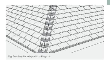
Fix remaining batten brackets equally over the length of the hip, at maximum 600mm centres.
