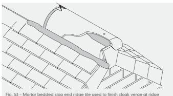
Fig. 53 – Mortar bedded stop end ridge tile used to finish cloak verge at ridge
