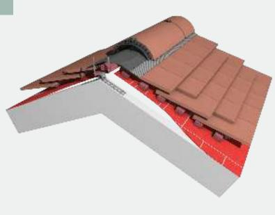
RidgeFast is a simple and rapidly installed, dry fixed ridge ventilation system suitable for all duo- pitch roofs using all Marley tile and slate profiles, as well as those of other manufacturers.
