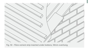
2 Commence laying an under eaves course of tiles using a standard eaves tile or a cloak verge tile cut down to size (Fig. 51, page 66). Where possible use a standard eaves tile, but establish what will be required for the top course at the roof apex, to ensure that the same unit is provided on both sides of the apex. In this way, opposite gable ends can be constructed with cloak verge tiles in different courses, but will still maintain a balanced appearance when viewed from the ground.
