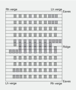
Fig. 1 – Loading roof evenly with tile/slate stacks
