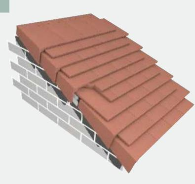
Plain tile cloak verges provide a weatherproof and mortar free finish to the roof verge. They are available in right and left hand units in colours to match the main roof tiles, twice nailed for maximum security. The apex of the roof is finished with matching stop-end ridge tiles.
