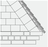
Fig. 34 – Fixing tiles to raked batten
