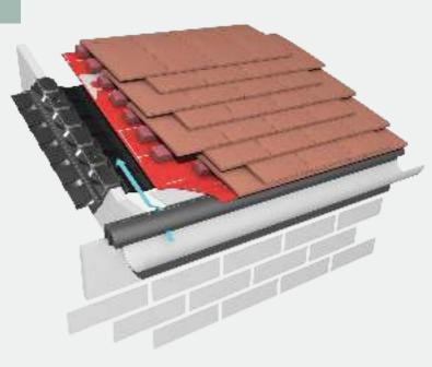
Marley Universal eaves ventilation systems are designed to provide continuous 10mm or 25mm free vent areas to roof voids in an efficient and unobtrusive manner for roof pitches from 12.5° to 55°. The 25mm system can also be used to ventilate the batten cavity where this is required.
