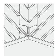
Fig .66 - Construction of valley boards
