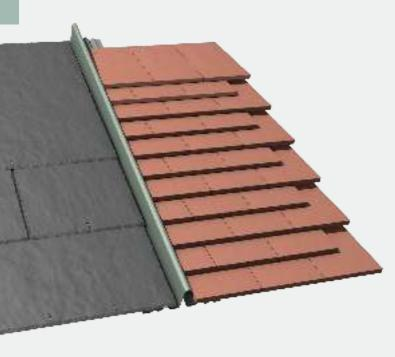
Mortar-free, BS 5534 compliant weather-tight joins between dissimilar roof coverings.
