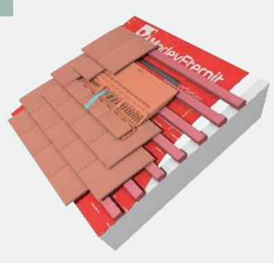
Available in a range of bases with real clay tile slips on the visible edge (3 tiles wide). The clay tile vent provides a net ventilation area of 7,500mm² per vent. Suitable for natural, mechanical or soil pipe ventilation.
