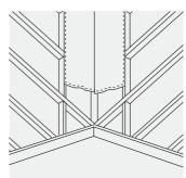
Fig. 67 – Butt joint valley boards over supporting rafters
