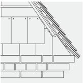
Fig. 33 – Cut tile to meet rake of verge
