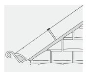
Fig. 16 - Bedded and mechanically fixed third round third hip ridge tiles used as hip capping with hip iron
