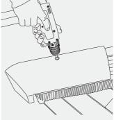
Fig. 61 - Fixing Third Round End Hip tile
