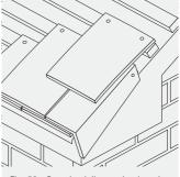
Fig. 52 – Standard tile used to break bond
