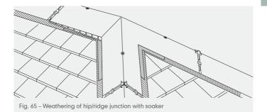
14 Where Marley RidgeFast is also being used and the hip tiles are the same as the ridge tiles, a Tapered Filler unit must be fitted beneath both edges of the end ridge tile to ensure a close fitting mitre can be achieved at the apex (Fig. 65).
