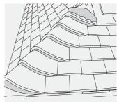
Fig. 17 – Bedded and mechanically fixed bonnet hip tiles
