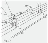
To establish the appropriate point at which to bend legs of ridge batten bracket and depth of ridge batten (1 or 2 tiling battens), Temporarily secure a short length of top course tiling batten and loose lay top course tiles either side of ridge. Position a ridge tile centrally onto roof tiles. By offering up a ridge batten bracket to the side of ridge tile bend point and batten thickness can be assessed so that minimum 20mm screw penetration is achieved.
