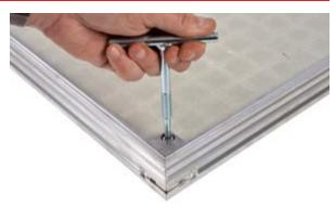
**Step 2:** Unscrew and remove the locking screws with the lifting/locking keys provided. Take care when unscrewing the locking screws on ASSIST versions as the cover may start to open automatically once the screws are unfastened. If this happens simply hold the cover in place until ready to be fully opened.
