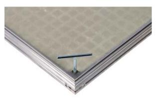
**Step 3:** For recessed covers use at least two lifting/locking keys and insert the threaded section of the key into diagonally opposite locking positions (ASSIST versions insert keys into locking positions on the opposite side to the hinges). Screw in both keys evenly until the cover raises slightly. Apply one more full turn to each key. The cover is now ready to be opened/lifted.
