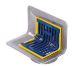
ACO Two Way outlets are located at the junction between flat roof and parapet wall providing "through the wall" drainage to external rainwater pipes and hoppers. Outlets are parallel threaded for connection to taper male, screw threaded adapters to ensure a completely watertight connection to pipes with 55mm, 82.5mm and 110mm outside pipe diameters.
