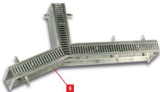
Integration of the rainwater down pipes was achieved without need for additional site-work through fabrication of special corners which included the required branch unit (3).
