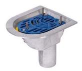
ACO Balcony outlets are designed to be installed against an abutment wall and permit the introduction of successive rainwater pipes discharging from higher level balcony areas. Balcony outlets are suitable for connection to pipes of 82.5mm and 110mm outside pipe diameters.
