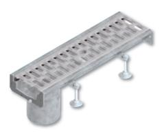
Shallow invert surface drainage system, manufactured from hot-dipped galvanised steel to BS EN ISO 1461:2009. Grating choice includes galvanised steel perforated, slotted and composite black and white to Load Class C250 to BS EN 1433. All gratings supplied complete with locking.
