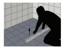
Remove the grating plastic friction locks from both ends of the grating and insert the LED modules ensuring the LED's are facing towards the centre of the grating and that the slightly angled face of the module is uppermost in the grating to allow water to drain freely.
