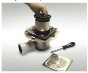
Remove crosshead screws from grating. Using appropriate gloves, grip the crossbar of the foul air trap and pull upwards making sure that the rubber sealing ring does not dislocate and fall into the drain. Remove sealing ring. Clean foul air trap thoroughly with soapy water.
