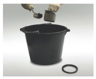
2. Lubricate the sealing ring with petroleum jelly and carefully locate the ring back onto the foul air trap. Lubricate the gully body in the area where the sealing ring will locate. Push the foul air trap firmly into position making sure that the trap seats squarely and that the sealing ring remains in position. Replace grating and tighten until resistance is felt.
