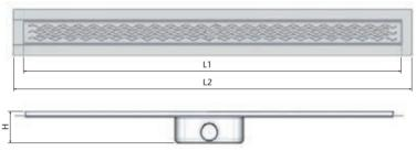
H = 92 mm with standard FAT (water seal height 50 mm)
