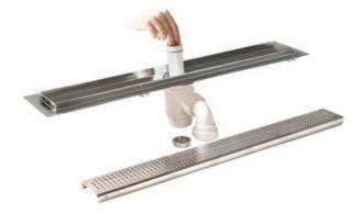
2. Simply pull the drain strainer out. The foul air trap can be removed by turning 1/4 turn anti-clockwise, and pulling out. Clean thoroughly with soapy water. Re-insert by lubricating the sealing ring with petroleum jelly, pushing the trap firmly down and twisting 1/4 turn clockwise. Check full location by gently pulling upward. Replace drain strainer, the grating is re-inserted by pressing down evenly into the channel.
