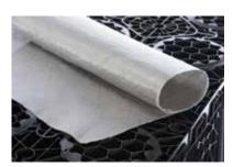
A polypropylene permeable nonwoven geotextile, for use in infiltration applications. ACOTex permits the passage of water into and out of ACO StormBrixx system, and also prevents the entry of sediment into tanks incorporating sediment forebays.
