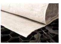
Manufactured from polypropylene this thick non-woven protection fleece is used to protect a geomembrane from mechanical damage due to ground and thermal movement. The protection fleece is placed on the outer side of the geomembrane. ACOTex Plus can be used with ACOWrap or with a welded geomembrane system.
