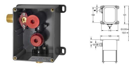
Basic installation kit for FLUSH-C manually operated and FLUSH-S non-touch, opto-electronically controlled urinal flush valve DN 15 for installation in walls. With wall mounting box and function block with integrated lockable water quantity regulator as well as remove plug for flushing and pressure testing.
