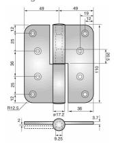
Allows symmetrical routing. Supplied with 8 wood screws.
