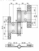
Supplied with 8 wood screws. (Dimension drawing shows RH hinge.)
