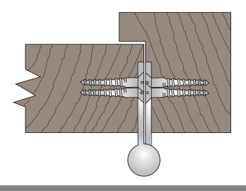
Use only the ASSA screws provided when fitting hinges to timber doors, as the load-carrying capacity of the hinge is dependent on the correct screws being used. A pilot hole should be drilled for the screws. ASSA hinges are normally supplied with 10g wood screws: we recommend preparing the pilot holes with a 2.4mm diameter drill.
