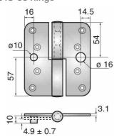
Allows symmetrical routing. Supplied with 8 wood screws. Integral 10mm diameter security dog bolt.
