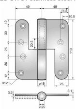
Supplied with 8 stainless steel fully threaded wood screws. Hinge, including journal pin, constructed entirely from stainless steel.
