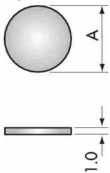
May be inserted into the hinge knuckle to raise the door.
