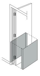
Large size formed angles for protection of door edges and faces.
